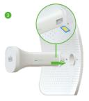
3. Insert the Micro SIM card and close the Radio Feed into the Feed Receiver
